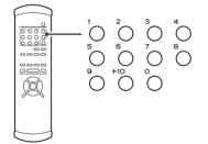
Use the number button to select tracks for playback. Use the +10 button to enter the first digit of numbers greater than 9 (repeated presses show 1-, 2-, 3- etc.) and the single digit buttons (0 through 9) for the second digit, or single-digit track numbers.
